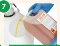
Fill vessel with BOK and top up with water
