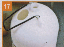
17 Empty & rinse vessel, fill with water & reconnect
