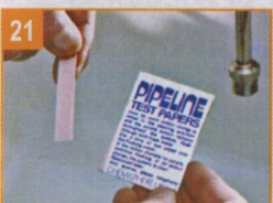
21 Check rinse water with test papers Blue = Pipeline present Pink = Rinse complete
